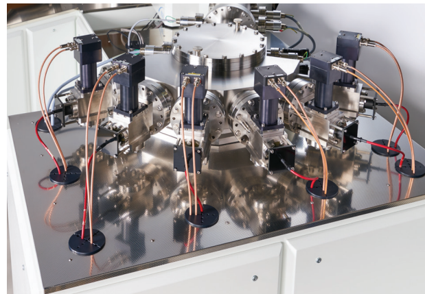
Multiple Daly detectors on a standard Plasma 3
